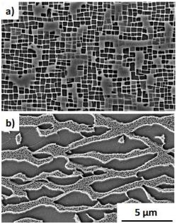
Microstructure of CMSX-4SLS (1 at. % of Re) a) Before creep test b) After creep test at 1150 °C / 90 MPa
