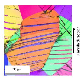
EBSD map of Ti-7Cr-1Al-1Fe (% wt.) during SEM in-situ tensile test Photo credit: Y. DANARD (Chimie ParisTech)
