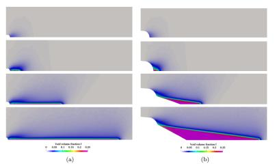
Crack extension in (a) initial (b) deformed configurations in an Infinite Medium (boundary layer model)
