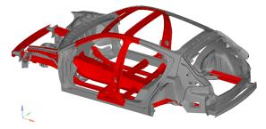
Typical applications of Press Hardened Steels in a Body-in-White structure
