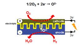
$H_2 + O^{2-} \rightarrow H_2O + 2e^{-}$ Architectured electrode/electrolyte interfaces in a SOFC technologie
