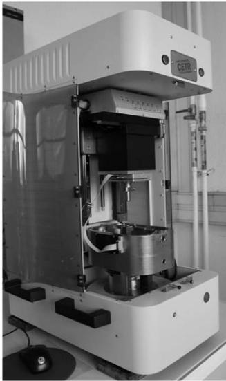
It is a flexible instrument for linear reciprocating to measure wear and fretting behaviour of a wide range of materials, including ferrous and non-ferrous metals, plastics, ceramics, paper,
